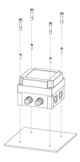
SP151 should be mounted vertically, and the cable should be connected upside down to avoid water from seepage. ▼ SP151 sealing ring has 4 mounting holes with center to center spacing of 113.5 × 113.5 mm.
